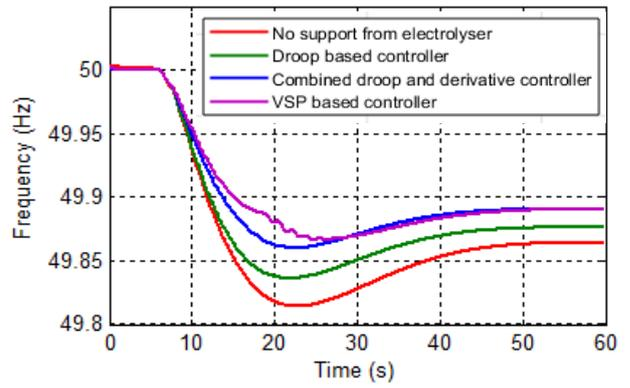
Figure 10. Frequency Response from electrolyser due to FAPR controllers
