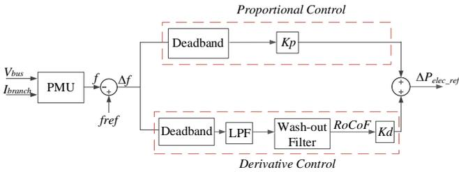
Figure 6. Combined droop and derivative-based FAPR
