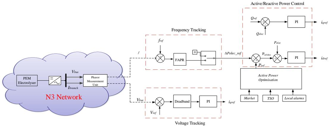
Figure 3. Outer controller structure of PEM electrolyser
