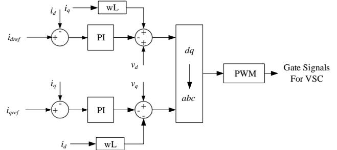
Figure 4. Inner controller structure of PEM electrolyser
