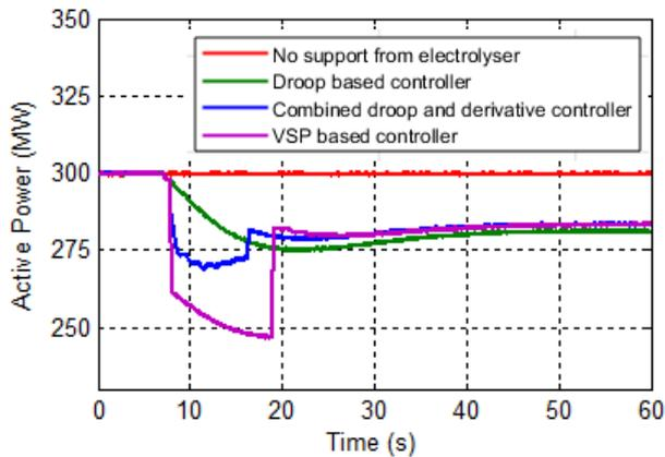
Figure 9. Power Response from electrolyser due to FAPR controllers
