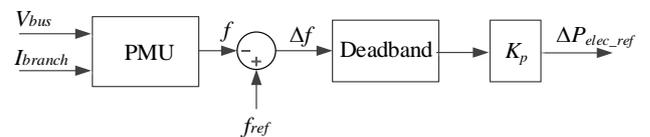
Figure 5. Droop based FAPR controller.
