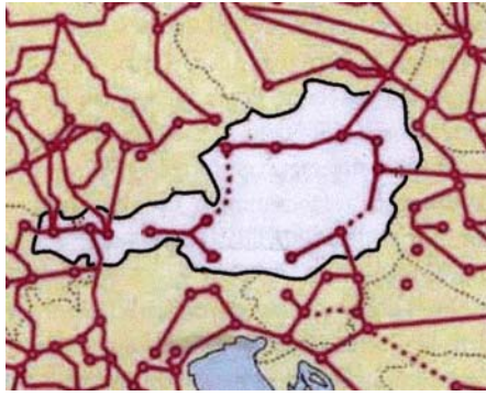
Fig. 1 The Austrian high voltage 380kV grid, (Fischer-Drapela, 2003)
