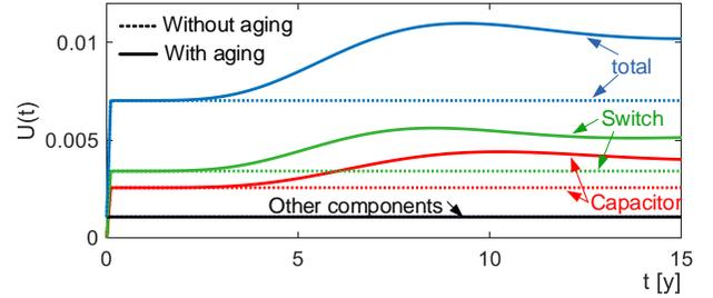
Fig. 12. Impact of component aging on the converter unavailability,  $U(t)$ ;  $(\alpha, \beta)_{\text{switch}} = (12, 3)$ ,  $(\alpha, \beta)_{\text{cap}} = (10, 3)$ .
