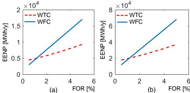
Fig. 15. Impact of WTC and WFC unavailability (FOR) on the EENP by the (a) 40 MW and (b) 160 MW WF.
