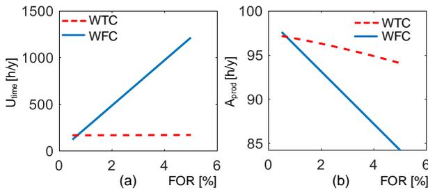
Fig. 14. Impact of WTC and WFC unavailability (FOR) on the (a) time-based unavailability and (b) production-based availability of the WF.
