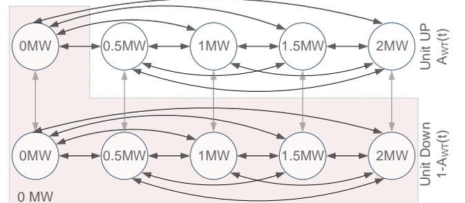
Fig. 6. A 2 MW WF reliability model – the highlighted states show zero generation.
