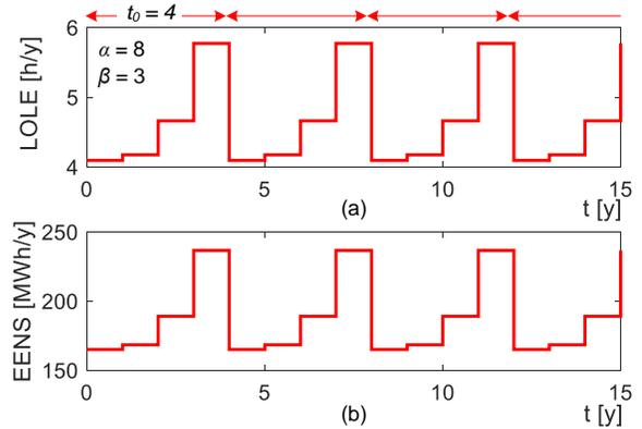
Fig. 20. Impact of the age replacement policy of HC on the reliability of FE-RBTS with 160 MW WF, (a) LOLE, (b) EENS.
