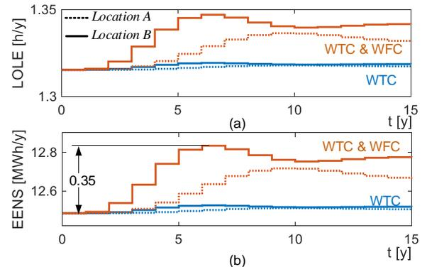
Fig. 16. Impact of WTC and WFC wear-out on the reliability of RBTS with 160 MW WF, (a) LOLE, (b) EENS.
