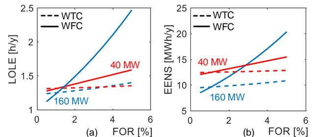
Fig. 17. Impact of WTC and line converter unavailability (FOR) on the (a) LOLE and (b) EENS in RBTS with 40 MW and 160 MW WF.
