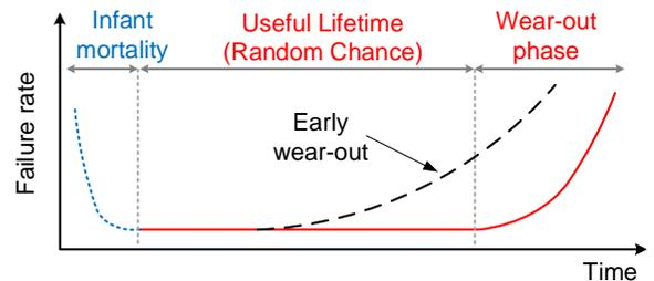
Fig. 1. Typical failure shape of an item known as bathtub curve.
