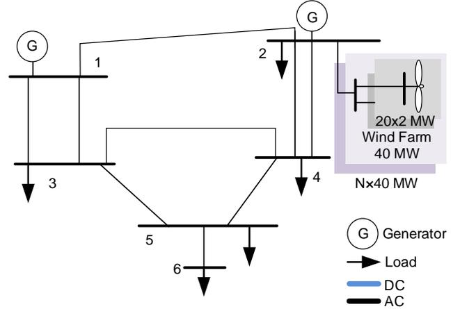
Fig. 8. Modified RBTS (The main version is provided in [57]), Wind Farm Converter (WFC).
