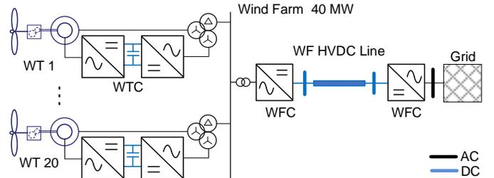
Fig. 9. A 40 MW DFIG based Wind Farm (WF) Structure with  $20 \times 2$  MW Wind Turbines (WTs).
