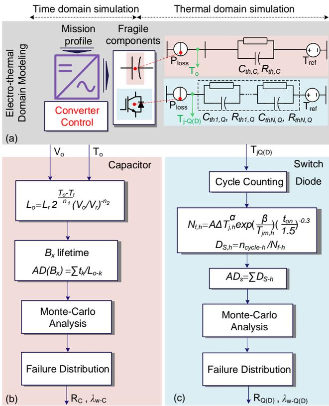
Fig. 2. Wear-out failure rate prediction in power converters, (a) electro-thermal mapping, (b) wear-out failure rate of capacitors and (c) wear-out failure rate of semiconductor devices.
