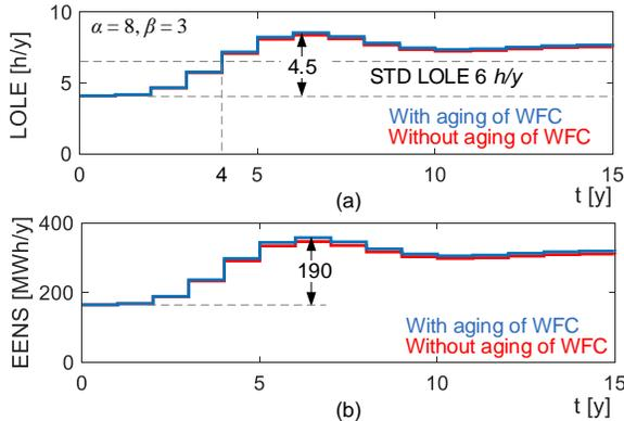
Fig. 18. Impact of WFC and HC wear out on the reliability of FE-RBTS with 160 MW WF, (a) LOLE, (b) EENS.
