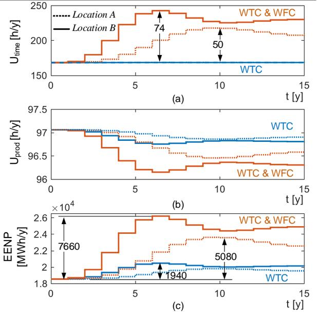
Fig. 13. Impact of WTC and WFC wear out on the reliability of 160 MW WF, (a) Time-based unavailability, (b) production-based unavailability, (c) EENP due to the wear-out of WFC or WTC.
