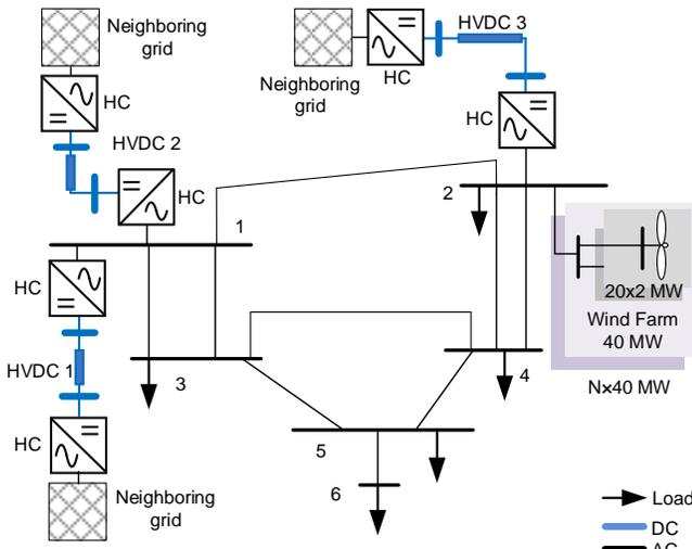
Fig. 11. Full Power Electronic based RBTS (PE-RBTS). HC: HVDC Converter.
