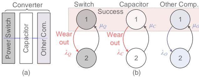
Fig. 4. Power converter reliability model; (a) reliability block diagram, (b) Markov model.
