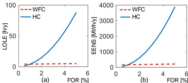
Fig. 19. Impact of WTC and WFC unavailability (FOR) on the (a) LOLE and (b) EENS in PE-RBTS with 40 MW and 160 MW WF.
