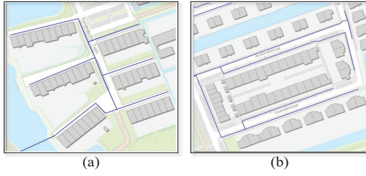
Fig. 2. Two deployment styles of cables in LVDNs.
