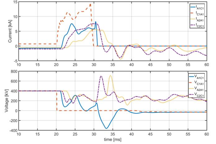
Fig. 8. Currents and voltages measured by critical relays
