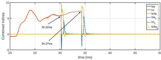
Fig. 13. Currents of DCCB1 with different delays
