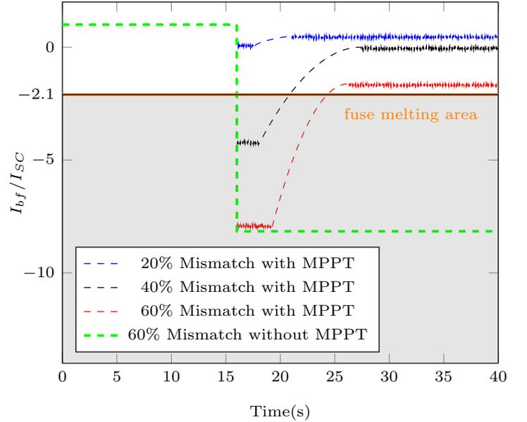
Fig. 3. Back-feeding current with different mismatch.
