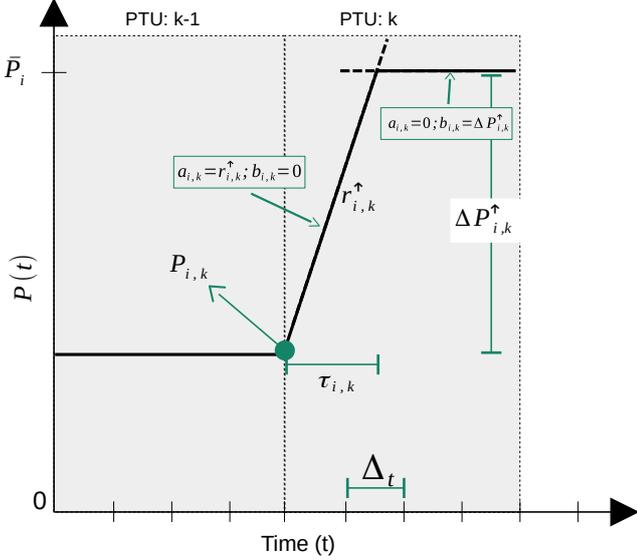
Figure 2: The sub-PTU power profile for resources with short time to ramp  $\tau_{i,k}$ .
