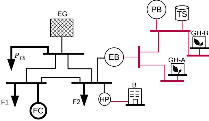
Figure 4: Proposed multi-energy system setup representing the FSP’s portfolio. The red area represents the heat network while the black part represents the electricity network.
