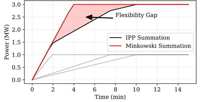
Figure 3: Aggregated portfolio power profile generated using Minkowski Summation method and IPP Summation method. The shaded region is the Flexibility Gap. The gray lines indicate IPP for R1, R2, and R3.
