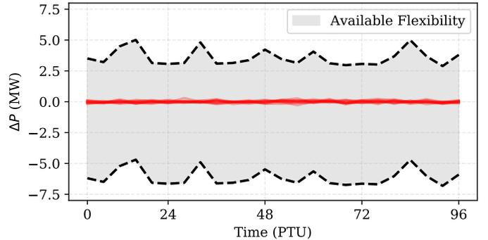
Figure 5: Assessing flexibility using Minkowski Summation. The red lines indicate the FR signal scenario set. The black dashed lines indicate the upper and lower levels of allowable power excursion calculated using the Minkowski method. The available flexibility bound is calculated in each PTU for the next PTU.
