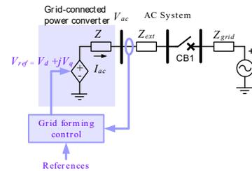
Fig. 3. Equivalent model of grid-forming converter using VSC.
