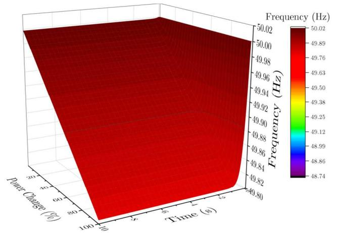
Fig. 9. System frequency response following the of SynC.
