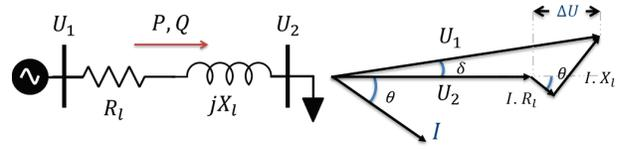
Fig. 1. Phasor diagram for a 2 bus system
