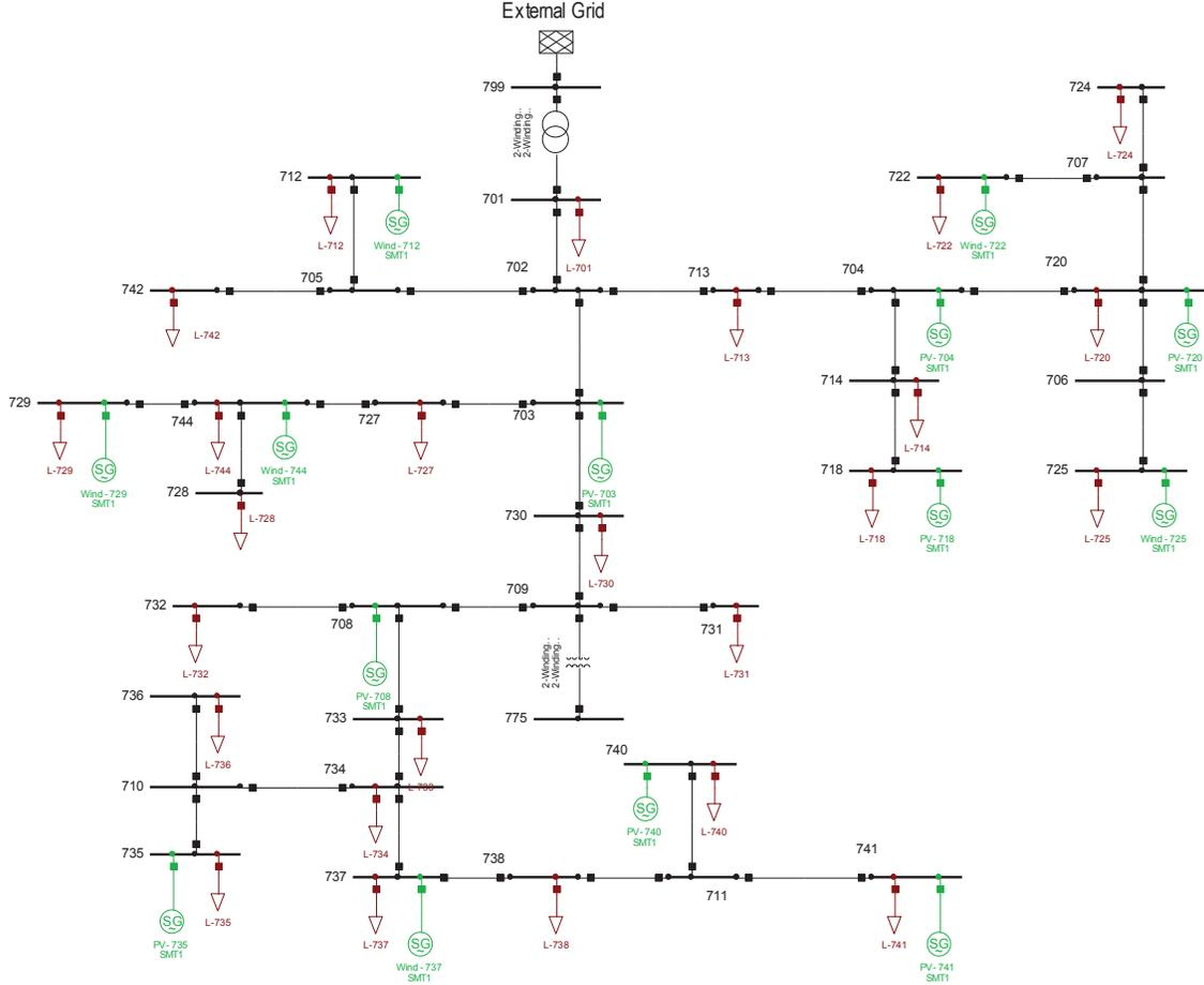
Fig. 2. The modified IEEE 37 node test feeder
